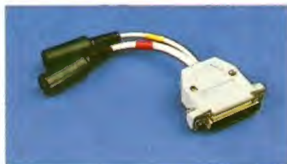
This interface plugs in to the Amiga and controls the video recorder: either via a LANC socket or the 'magic wand' remote control gadget.
